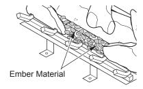
Figure 50 - Placing Ember Material on Burner
